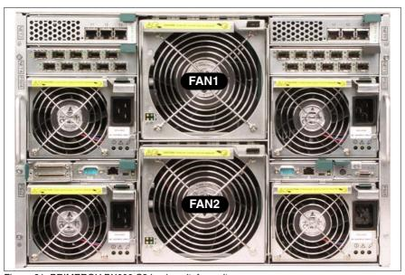
Figure 81: PRIMERGY BX600 S3 basic unit: fan units
